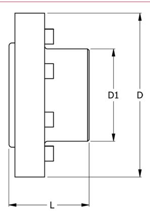
D = 180 D1 = 125 L = 80 Max bore = 75 Torque (N m) = 880
